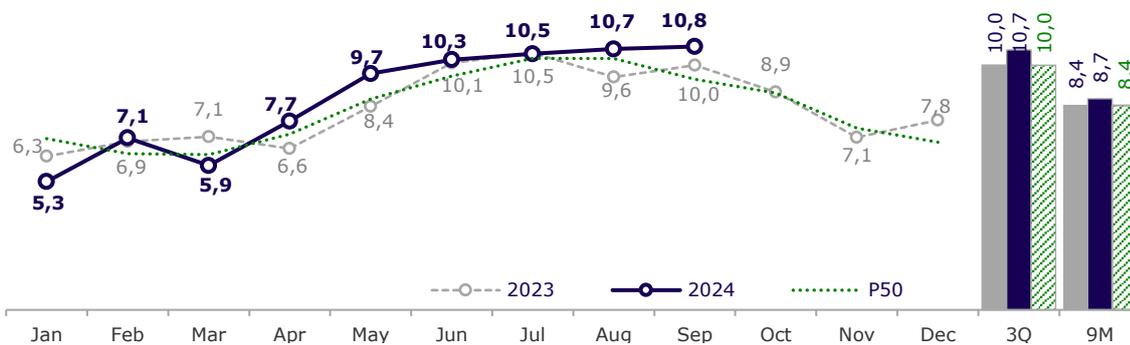
Assessing the results of 3Q24 based on the technical parameters of the project, winds were 1.8% above the long-term average. The performance of the wind turbines was 2.7% above expectation due to the high availability of the asset, while the performance of the farm’s power grid was 1.0% above expected. Curtailment negatively affected the quarterly results by 4.4%.
