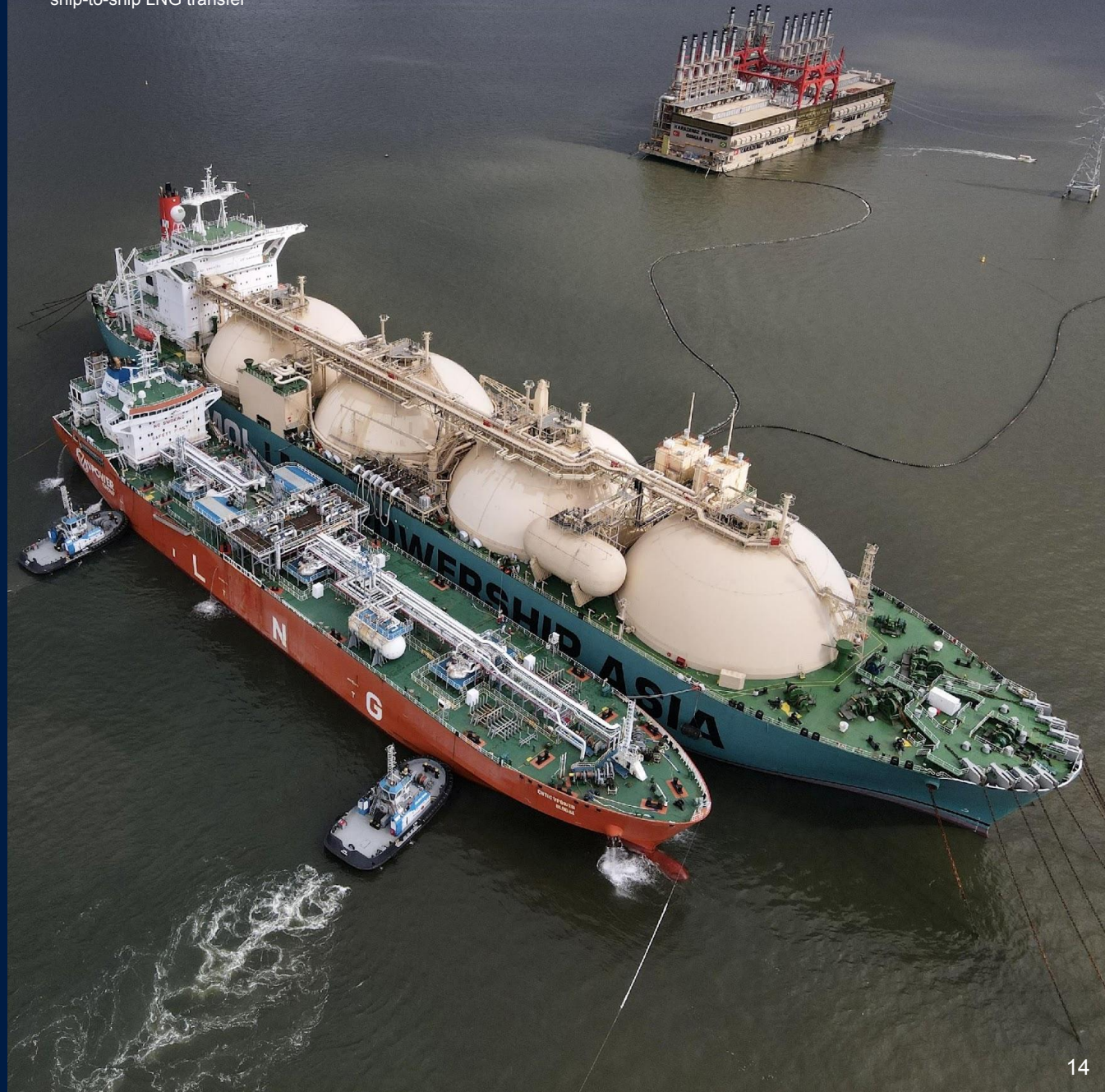
WS tugs assisting a ship-to-ship LNG transfer
