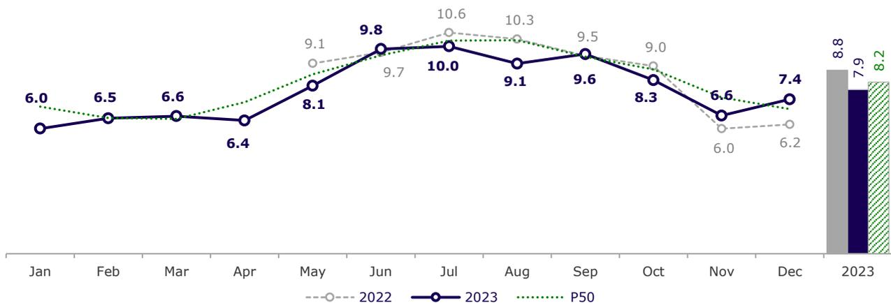
Assessing the results based on the technical parameters of the project, in 4Q23 winds were 1.9% below the long-term average for a 20-year horizon (estimated period of power generation based on P50). The availability of wind turbines, in turn, was 0.9% above expected, while the performance of the complex's power grid<sup>18</sup> was 0.3% above expected. Generation restrictions negatively affected the quarterly results by 0.9%, of which 0.4% can be reimbursed.
